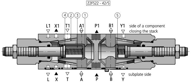
Hydraulic fluid from the port **A** flows through the throttling slot (1) to the receiver. At the same time, the fluid under operating pressure flows through port (2) to the side (3) of the piston (4) which is loaded with the spring. The piston (4) is therefore maintained in the
