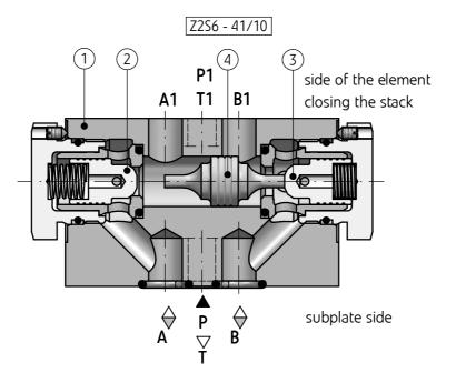
Pilot operated double check valve type Z2S6... is made by fitting two pilot operated check valves (2) and (3) in one housing (1). There is a free flow from A1 to A or/and B1 to B while from A to A1 and/or B to B1 flow is blocked. When, for example fluid flows through the valve from A1 to A, the piston (4) is shifted to the right and pushes the poppet of the
